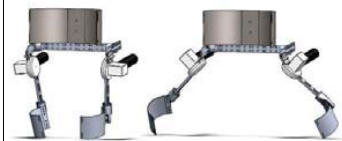
Fig.6 Open and close of the leg frame
