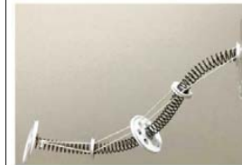
図10 意図しない方向に曲がる原因 Fig. 10 Cause of unintended directional bending
