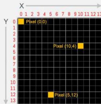
figure 6: X,Y Grid for a Display
